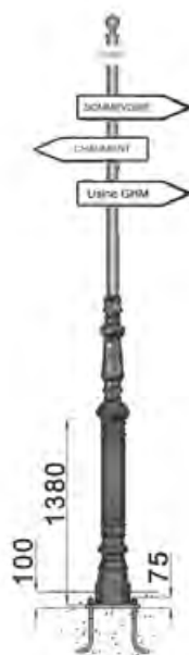
4 inserts Ø24x500 spacing Ø320 mm
